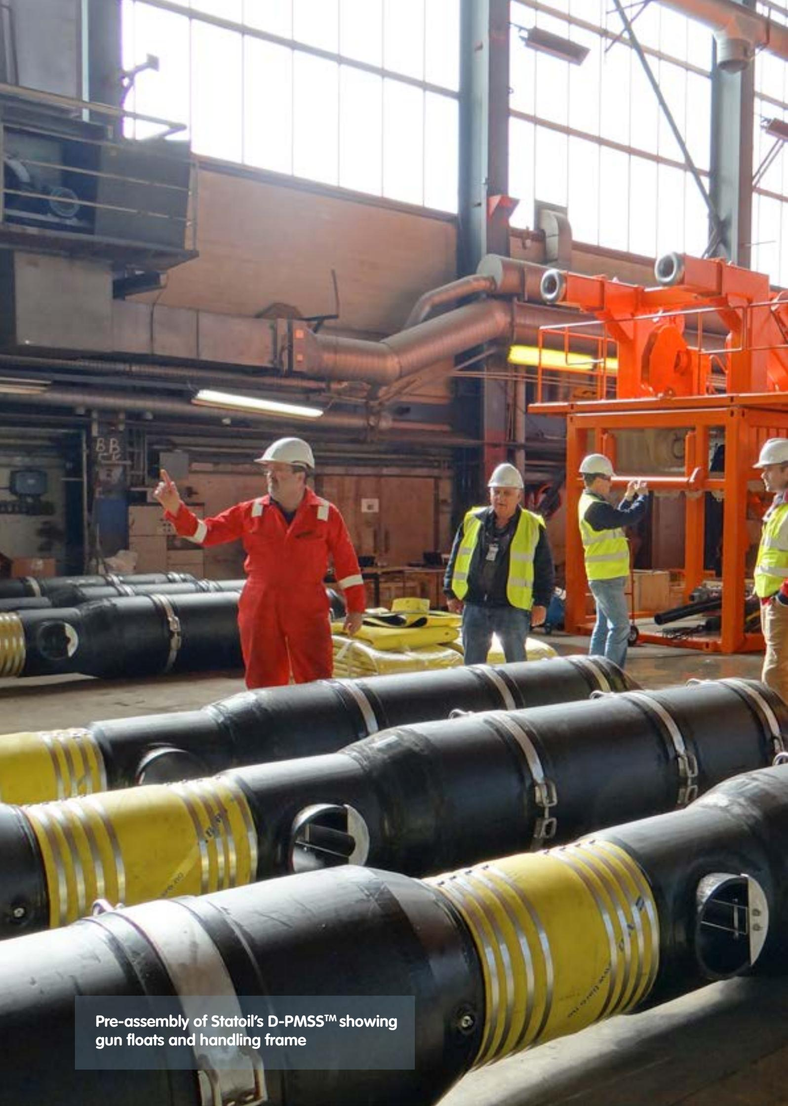
Pre-assembly of Statoil's D-PMSS™ showing gun floats and handling frame
